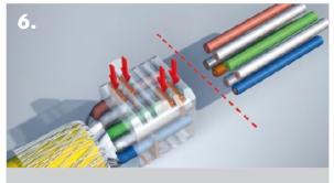
The installation tool securely presses all eight IDC contacts into the final position and also cuts the wire ends to the correct length. Assembly of the preLink® cable termination is complete.
